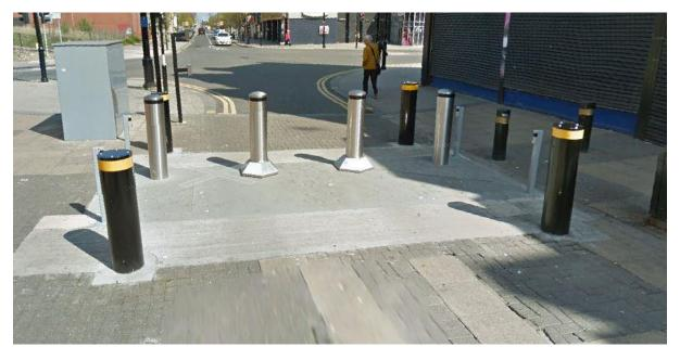
This sliding bollard system in South Shields includes additional black bollards which are not proposed for York.
